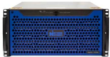
Note: The configuration tested had 192 TB of disk. The head unit contained a server system and the Network Instruments data capture cards. The main unit was connected to the three lower units and these provided additional storage capacity.
